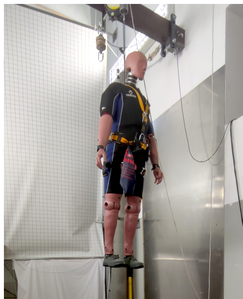
Figure 3. Fall from a height experimental stand. The two smartwatches are on the wrists of the dummy, and the tags are located on the belt. The bag in the front contains the Raspberry Pi and the batteries.
