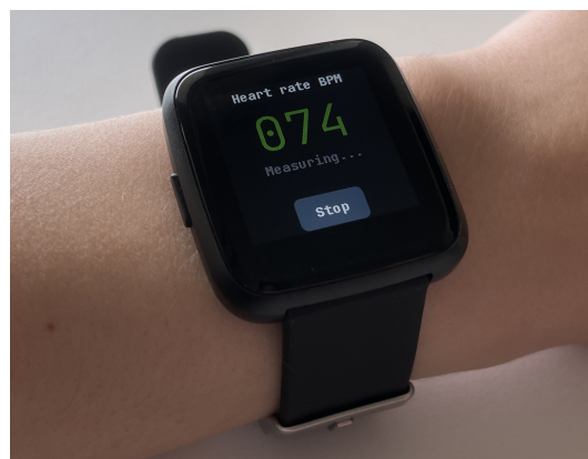
Figure 1. The PineTime smartwatch measuring the user's heart rate.
